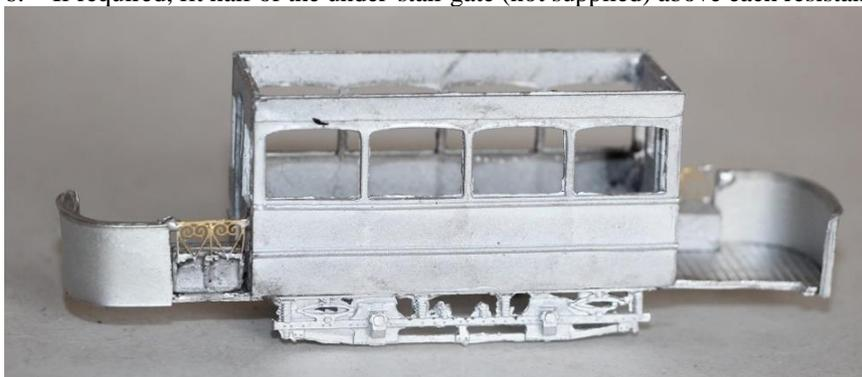
7. On a flat surface, solder the two halves of the upper floor together then fit centrally to the body.
