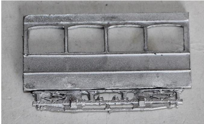
2. Produce the lower saloon box of 2 lower sides and 2 bulk heads by assembly on a flat surface in the upside-down position
