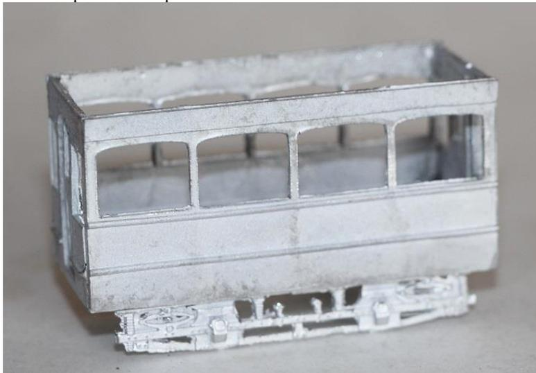
3. Attach the platforms centrally under the bulkheads with the rear wide sections flush with the bottom of the bulkhead. You will need to trim the edges of the platforms so that they fit inside the body.
