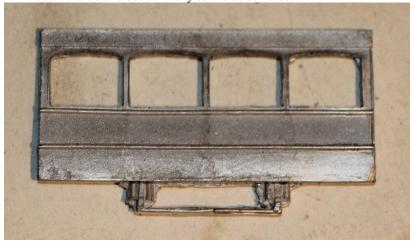
Produce the lower saloon box of 2 lower sides and 2 bulk heads by assembly on a flat surface in the upside-down position
