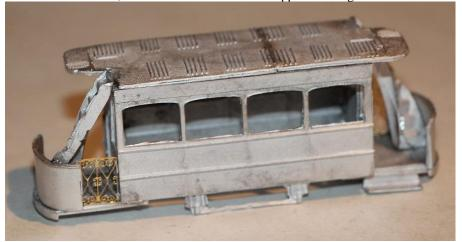
7. Fit the axle retainers to the lower floor (the wheels will be inserted once the lower deck has been painted), but don't fix in place until the interior is painted and the wheels are fitted.
