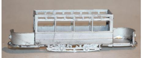
5. On a flat surface, solder the two halves of the upper floor together then fit centrally to the body.
