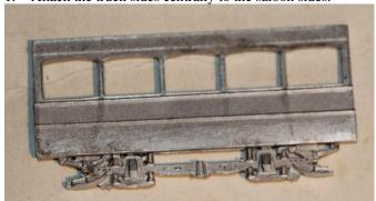
2. Produce the lower saloon box of 2 lower sides and 2 bulk heads by assembly on a flat surface in the upside-down position.
