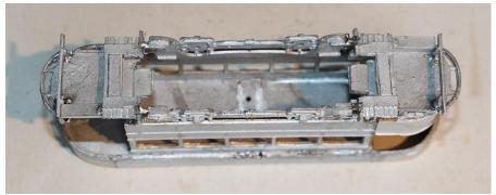
Fit the trolley mast to the left of the middle of the upper floor. Fit the stairs unless you wish to paint them first.
