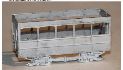
3. Attach the platforms centrally under the bulkheads with the rear wide sections flush with the bottom of the bulkhead. You will need to trim the edges of the platforms so that they fit inside the body.
