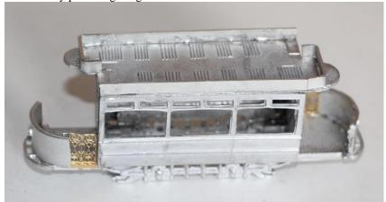
8. Turn model over to fit the steps, lifeguards and life trays. Fit the side lifeguards if required.
