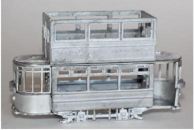
9. Fit the balcony ends, bending the end panels so that they match the shape of the upper floor.
