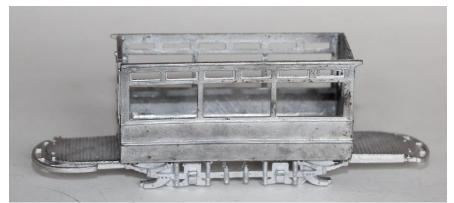
5. Gently bend the driver vestibule to match the curve of the dash. It fits with the blocked-in windows at the top.
