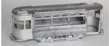
7. Fit the upper sides centrally to the sides of the floor so that they line up with the lower sides. Fit the upper bulkheads between the ends of the upper sides.
