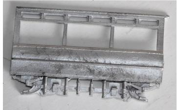
3. Fix one bulkhead square to each side, then join the two sub-assemblies together to create a box.
