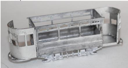
6. Fit the upper floor centrally to the body and flush with the drive vestibules.
