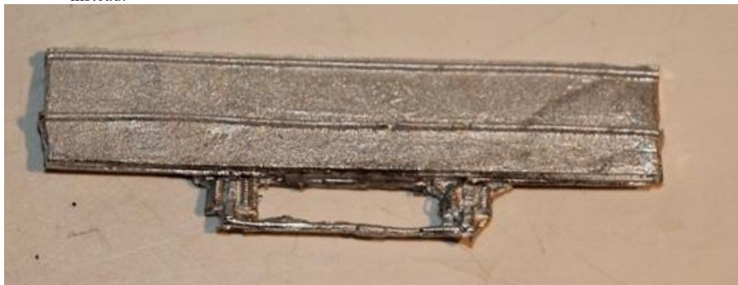
2. Fix one bulkhead square to each side, then join the two sub-assemblies together to create a box.
