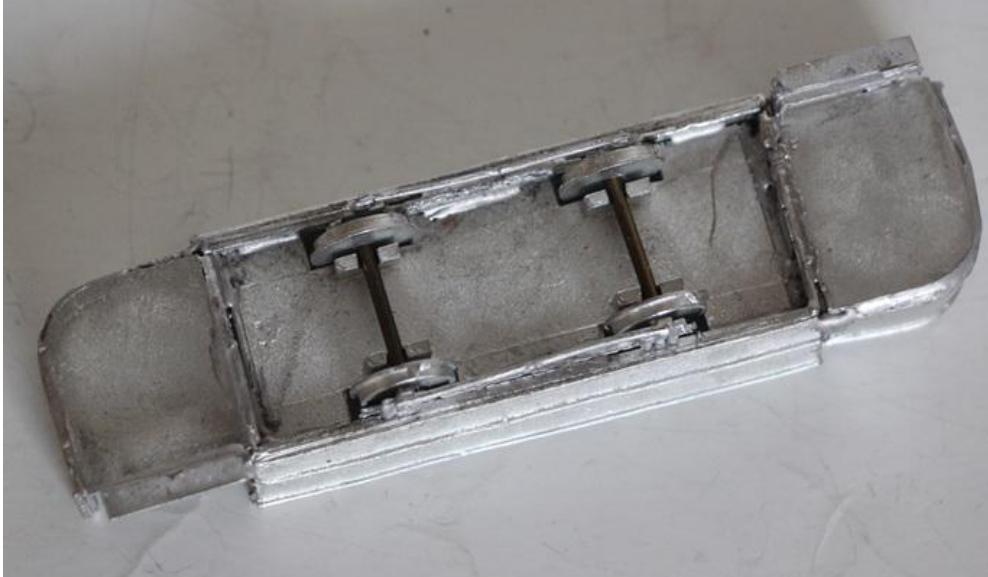
8. Cut the seating strip to create seats along the sides of the saloon. You may need to cut notches for the roof support wires.
