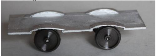
8. Turn model over and put the floor in place (do not fix it in place until you have completed the painting and glazing of the interior of the tram). Use the location of the wheels to fit the axle boxes in place. Fit the steps. Fit the brackets to the middle of the lower edge of the platform.
