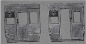
2. Fix bulk heads to sides squarely and marry subassemblies to produce a box effect.
