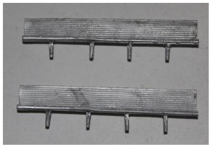
10. Take two of the double seats and the two single seats, and make them into 2 triple width seats. The seat backs are not required.
