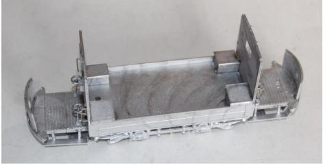
12. Solder the halves of the tanks together then fit the ends.
