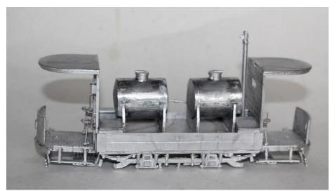
16. Make up roof supports and bulkhead supports and fit. Drill a hole in the trolley pole head and the trolley mast top. Cut brass wire to appropriate length and fix the trolley pole head to it, then fit to trolley mast head. Make up the trolley pole hook and fit.
