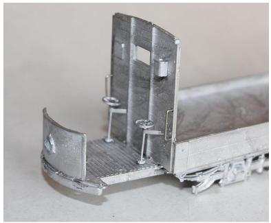
10. With model inverted, fit the steps, front lifeguards and the lifetrays, adjusting the height to suit the truck sides.
