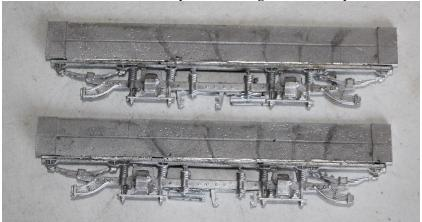
3. Make up handrails from wire and fit to bulkheads. Fit the conduit switch to the bulkheads to the right of the window.
