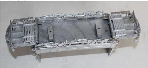
11. Fit the box fronts on the top edges of the sides adjacent to the bulkheads. Cut the box sides and backs down to suit the height of the floor. Fit to the sides to the outer edge of the fronts and the box backs behind them. Then fix the tops with the edge flush to the front.
