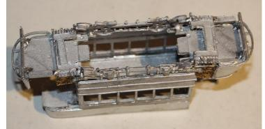
Fit the second under-stair gate against the edge of the bulkhead on the offside of the platform.
