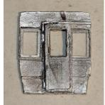
3. Produce the lower saloon box of 2 lower sides and 2 bulk heads by assembly on a flat surface in the upside-down position
