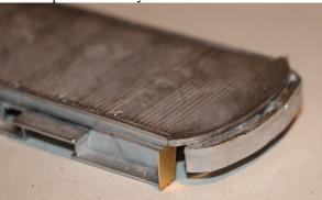
9. Fit the dash panels flush to the ends of the floor, you may need to bend them a little to match the curve of the floor.
