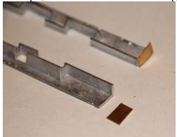
7. Fix the steps under the sides of the floor. The longer step should be fixed to the upper left and lower right, and then the shorter step should fill the gap. The steps should be fixed at an angle so that the steps themselves are horizontal.
