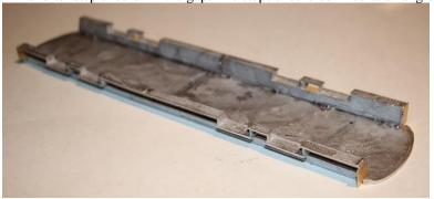
8. Fix platform ends / bumpers under the ends of the floor so that the platform end is flush with the end of the floor and the bumper extends beyond it.
