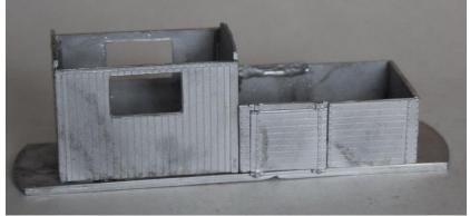
5. Remove the raised sections at the outside of the platform so that the dash fits well. Fit the platform end under the end of the floor. Fit the dash on top of the platform and against the end of the floor.
