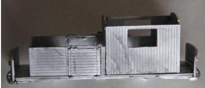
6. Remove the top edges of the truck sides so that it fits inside the edge of the floor. Fit the truck sides centrally to the sides.
