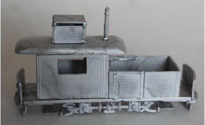
13. Fit the tower handrail supports on the inside of the tower platform fittings either vertically or at an angle depending on whether you want the tower handrail in a raised or lowered position.
