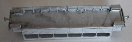
10. Fit the trolley planks to the roof, on the central line of the roof and with the outer ends flush with the ends of the sides. Don't fix the roof until you have painted and glazed the interior and fitted the seats.
