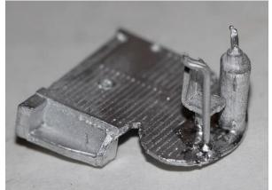
9. Fit the lifetray, side and end lifeguards under each platform. Don't fit the platforms in the car until the interior has been painted and glazed.
