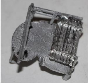
10. Fit the bumper flush to the bottom of the car end.
