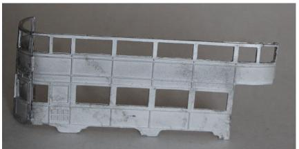
2. Trim the upper deck floor to fit, and fix to one end / side.
