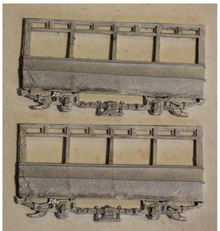
2. Fix bulk heads to sides squarely and marry subassemblies to produce a box effect.
