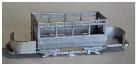
5. Fit the vestibules and windscreens. Start by fitting the windscreen centrally to the top of the dash. Take the nearside vestibule and remove the left hand vertical bar. Then bend the vestibule to fit. Fit the bullseye light in the top left window of the offside vestibule. Finally, remove the right hand vertical bar from the offside and bend that to fit.
