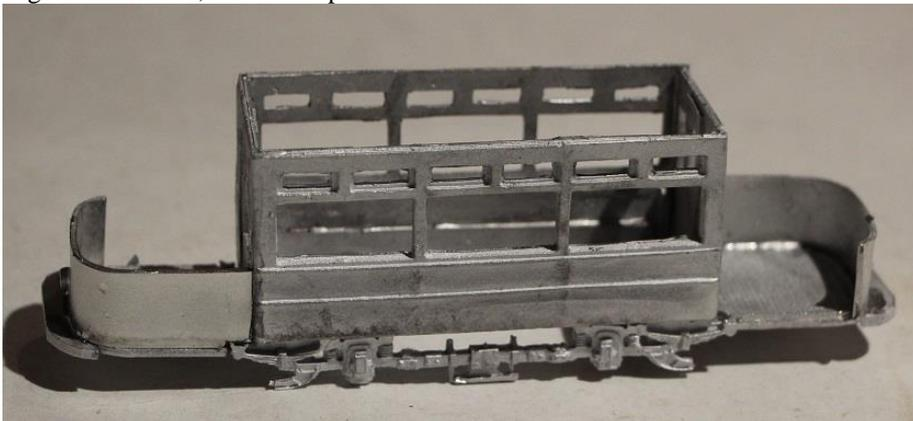
5. Fit the vestibules and windscreens. Start by fitting the windscreen centrally to the top of the dash. Take the nearside vestibule and remove the left hand vertical bar. Then bend the vestibule to fit. Finally, remove the right hand vertical bar from the offside and bend that to fit.
