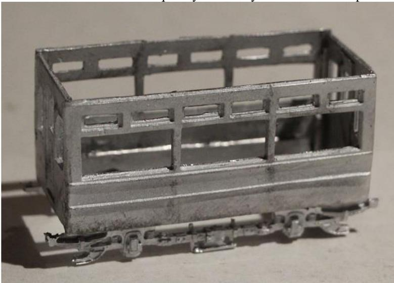
3. With model inverted, attach platforms to bottom edges of bulkheads with the rib inside the car saloon. You may need to trim the sides of the platform to make it fit inside the tram body and also to go behind the springs on the end of the truck sides.
