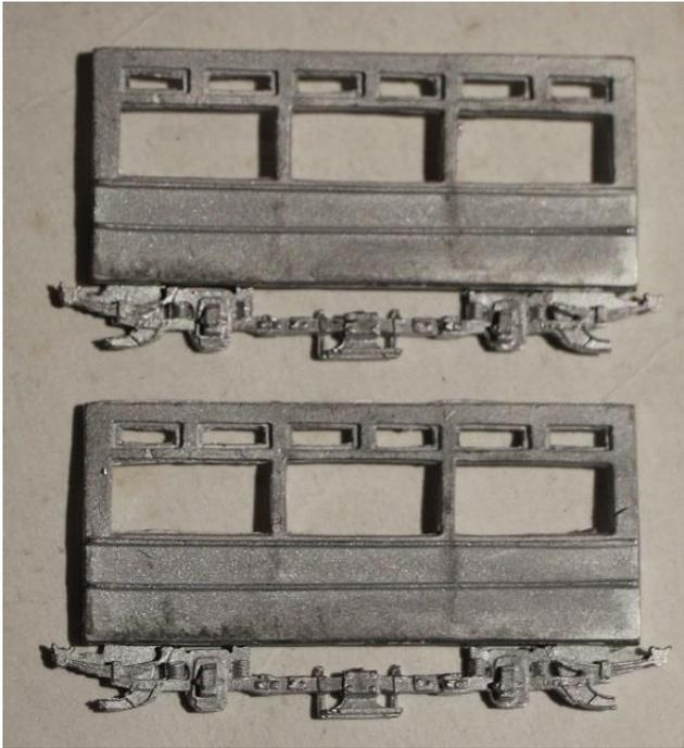
2. Fix bulk heads to sides squarely and marry subassemblies to produce a box effect.
