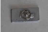
4. Fit the bogie top flush to the top of the base chassis.
