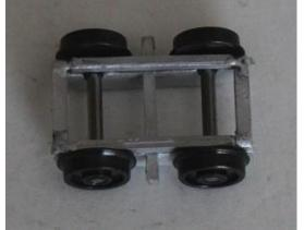
Fix the male half of the press stud into the centre of the bogie top. 3.
