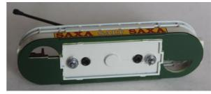
The lower deck floor should be removed by drilling a row of holes along each side of the body from underneath, through the lower deck seating and across both ends. These holes can be opened out, with a micro saw, into a slot to enable the floor to be removed. Then trim the ends back until the motor can be fitted.
