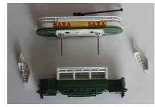
4. These rods also need to be removed from the upper deck casting by turning them and pulling at the same time or, on the open topped tram, by cutting them off with a saw.
