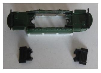
6. Fit the lifetrays and motor in the floor.
