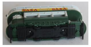
2. Each rod is surrounded by a plastic bush which, although not threaded, can be removed by pushing it round anti-clockwise with a screwdriver. The tram can then be separated. Retain all of the parts.
