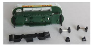
3. Separate the top and bottom halves of the tram.
