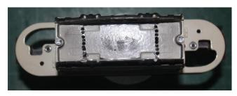
Now a piece of diecast floor has to be removed, first drill a hole about 1/8 th inch diameter in one of the small recesses in the floor. Then either elongate the hole with a file or drill a couple more holes in a straight line, so a junior hacksaw blade can fit into the hole. Take care not to
