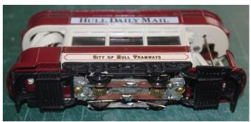
Drill off the rivets holding the lifetrays in place and remove them. Trim the ends so that they fit under the ends of the truck.
