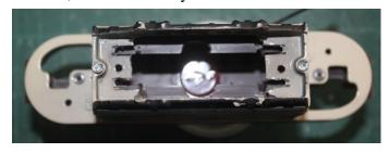
Enlarge the hole with a file to fit the motor, allowing room for the worms to turn freely.
