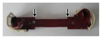
The platform casting should be cut where it narrows at the inner end of the platform.
