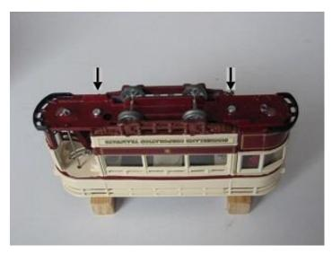
When the baseplate rivets are released the wheels, axles, lifeguards and platform handrails will fall out, the handrails and lifeguards should be placed in a safe place for use later.
