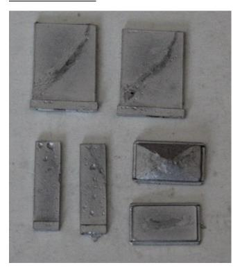
Assemble the front, back and two sides to form a box, with the sides inside the front and back. The beading should line up at the bottom
