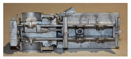
12. Cut the front axle to 29mm, and the rear axles to 32mm. Fit the front axle transmission shaft / diff (29) into the remaining hole in the front of the forward jacking frame and over the front axle. Fit the rear axle transmission shaft / diff (28) into the hole at the rear of the forward jacking frame and over the rear axles.
