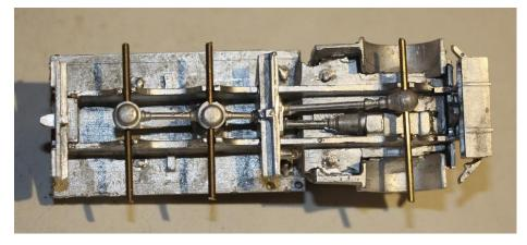
13. Fit the rear jacking frame (33) with the block on the back fitting into the rear of the chassis. Fit the required stabilising jacks (11 or 12) into the front and rear jacking frames. Fit the exhaust (46) with the pin on the silencer in the hole in the nearside lower edge of the chassis.
