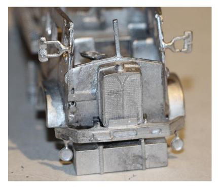
15. Fit the horn and warning lights (from sprue 52) to the cab roof, but don't fit the roof to the cab until you have painted and glazed the interior.
