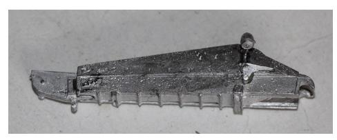
6. Fit the support frame (49) under the jib.
